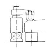
**Clamp** available with a tapped hole allowing the use of a wide variety of contact bolts or spindles, allowing for an increased clamping range.
