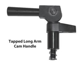
Long-arm Hook Clamps available with either a plain or tapped arm. The tapped-arm version accepts a wide variety of contact bolts or spindles to increase clamping-height range (the tapped arm is also slightly longer). Mounts in a reamed hole or in a Hook-Clamp Mounting Block or Holder (order separately). Ideal in tight spaces where high clamping force is required. Available in three sizes.
